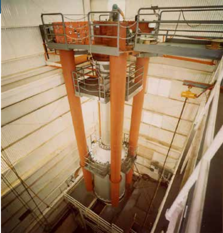
Fort St. Vrain Fuel Handling Machine (FHM)
